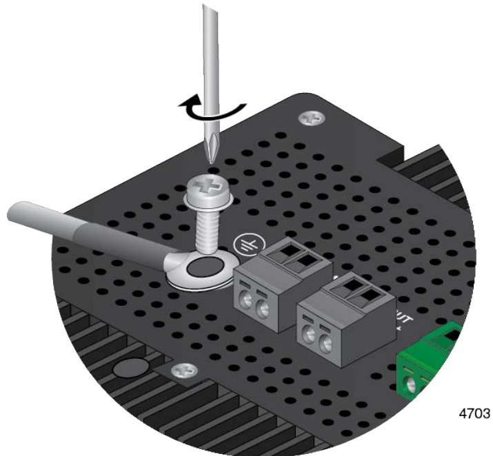
Figure 47. Attaching the Grounding Wire to the Switch
