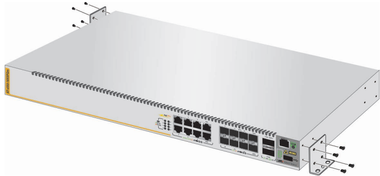
Figure 59. Installing the Brackets on the AT-x550-18XSPQm Switch
