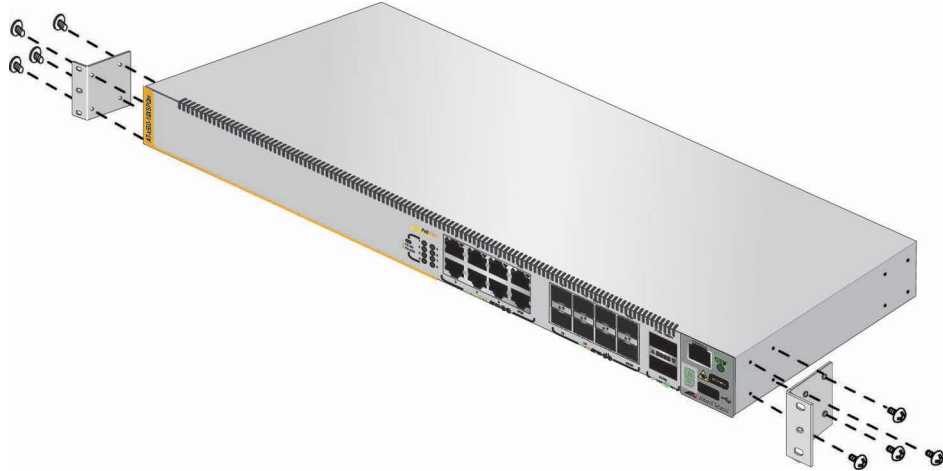
Figure 53. Example of Attaching the Brackets to the AT-x550-18XSPQm Switch
